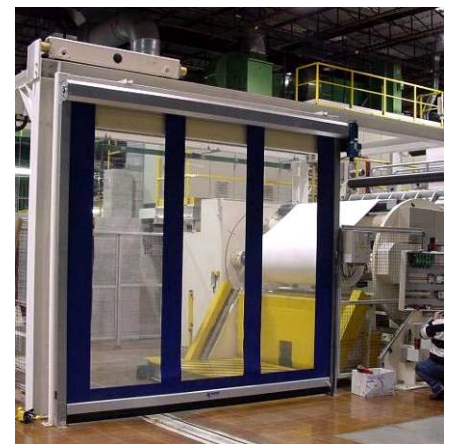
Fast-mode door for CE-safety compatibility
