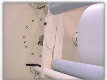
Rider rolls for optimization of the winding quality during reel change
