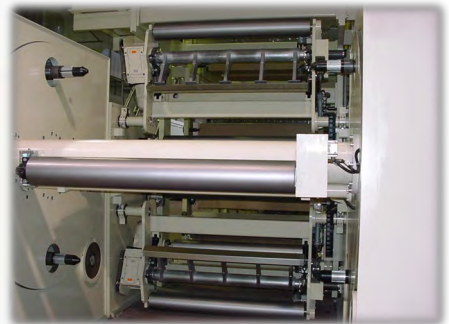
Two reel change systems TAC for reel change in both winding directions
