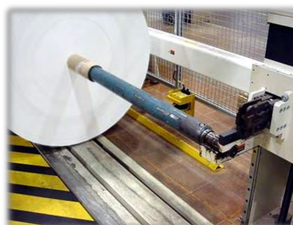
Winding shaft holder in combination with a floor conveyor
