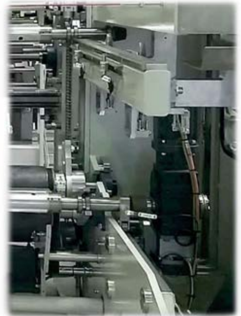
Winding slide with center drive
