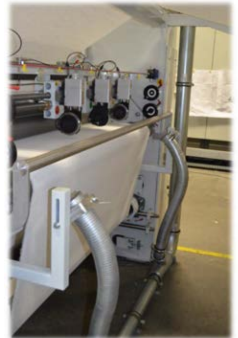
Edge trimming and slitting (scissors cut)
