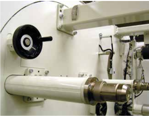
Spindle with manual adjustment by turning a knob
