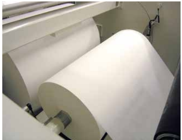
Reel change system with an active knife guidance
