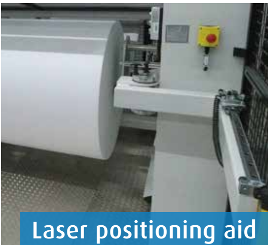
Swivel arm with precision-adjustable disk laser
