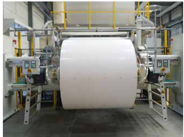
Shaftless winding station
