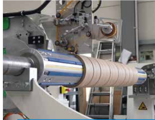
Winding shaft preparation with automatic application of adhesive
