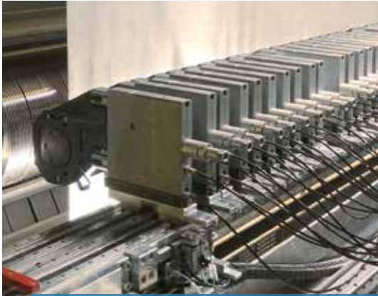
Slitters with the EPOS automatic positioning system
