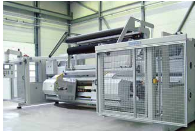
Shaftless winder for paper in a 3-metre working width
