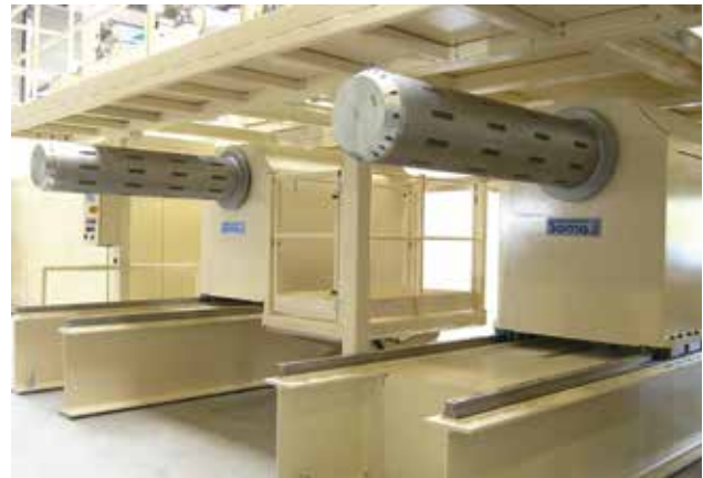
Unwinder for aluminium foil with an overhung winding shaft
